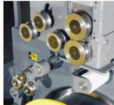
Pneumatic automatic end of coil roller, power feed head & wire rollers
