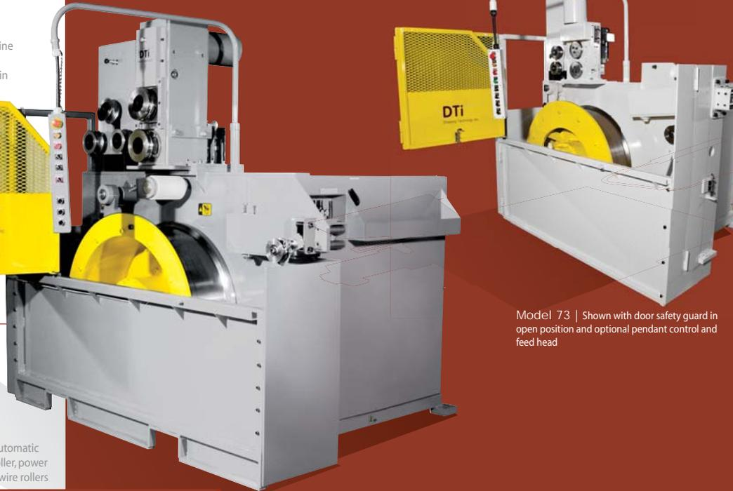
**Model 73** | Shown with door safety guard in open position and optional pendant control and feed head
