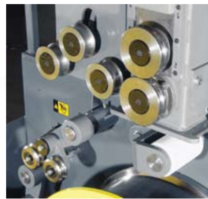
Pneumatic automatic end of coil roller, power feed head & wire rollers
